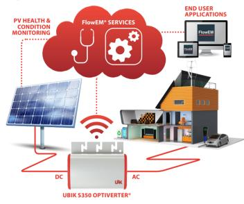
The UBIK S350 OPTIVERTER® has a **built-in Wi-Fi Interface**. This allows direct communication through any of the existing routers. Wi-Fi has been chosen as the most widely usable and reasonable communication solution for the end user.
