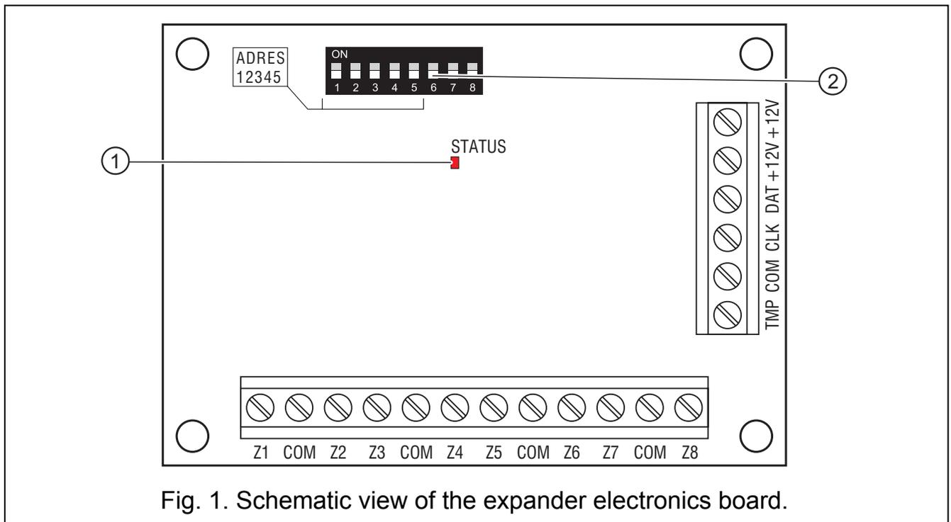
Fig. 1. Schematic view of the expander electronics board.
