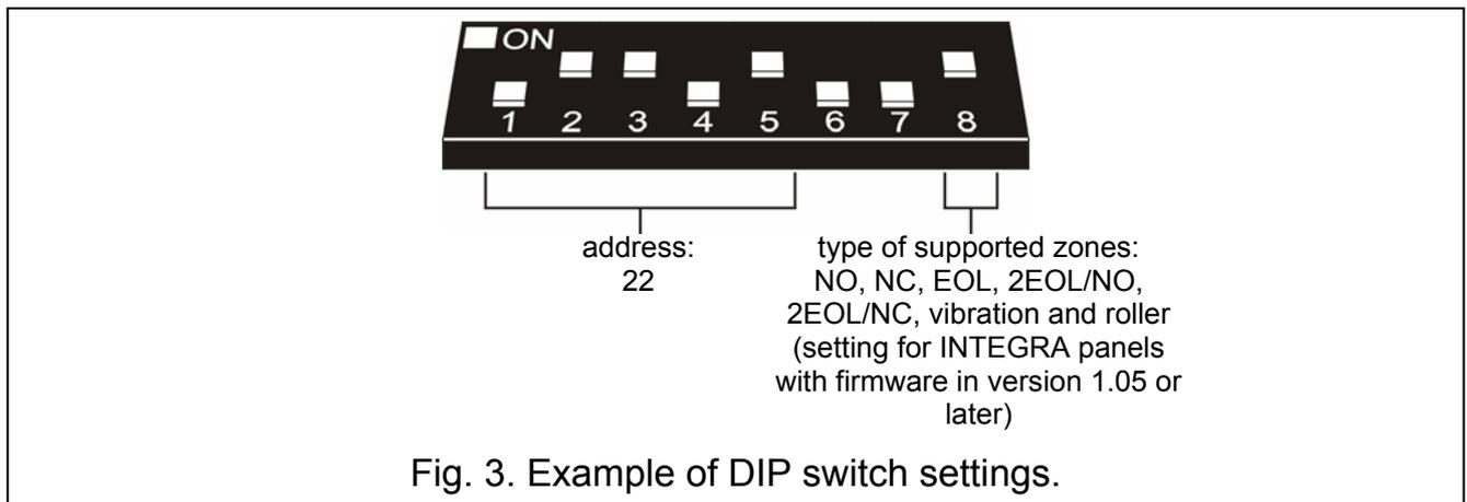
Fig. 3. Example of DIP switch settings.
