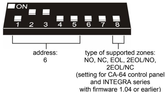
Fig. 2. Example of DIP switch settings.
